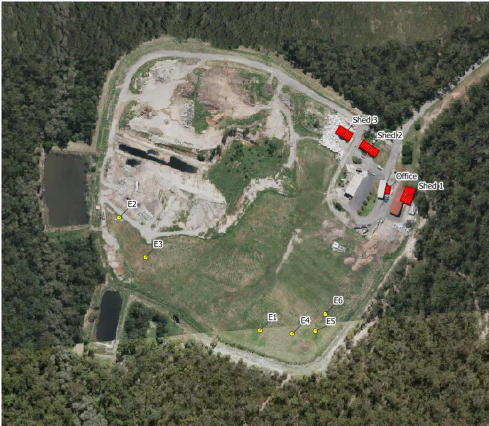
Figure 1: Surface Methane Monitoring – 5 July 2021 (Reported as Q4 in Table D4, Appendix D) (E1 to E6 – exceedances marked in yellow)
