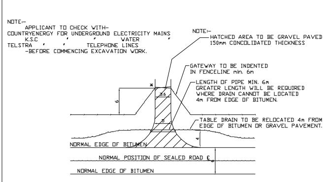
\* WHERE AN INTERNAL ROAD DIVERTS STORMWATER RUNDEF FROM WITHIN THE PROPERTY VIA A TABLE PRAIN TOWARDS COUNCILS ROAD RESERVE AN INLET PIT SHALL BE CONSTRUCTED WITHIN THE PROPERTY AND SUITABLY SIZED PIPE DIRECTED TO THE EXISTING TABLEDRAIN VITHIN COUNCILS ROAD RESERVE ON THE LOWSIDE OF THE PROPEDSED CULVERT. THE RELIEF PIPE SHALL BE SIZED IN ACCORDANCE WITH TABLE.
