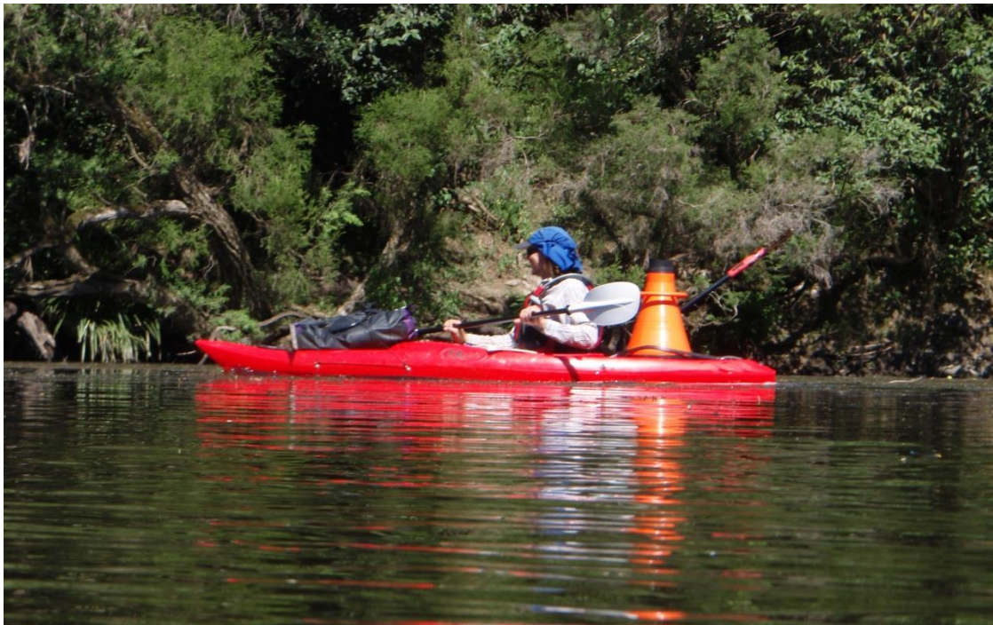
Figure 5 Macrophyte grapnel (wire brush attached to the end of a telescopic pole at stern of kayak) and bathyscope (orange cone at stern of kayak) used to assist macrophyte collection and identification in the field.
