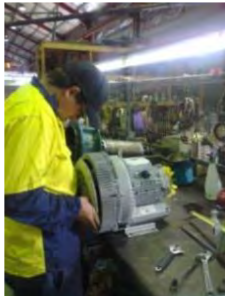
Carrying out routine maintenance on a sewer pump (above) and servicing the rainfall and river height telemetry canisters (below)
