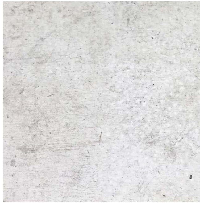
Concrete finishes (pathways and shelter slabs)- neutral grey with a light broom finish
