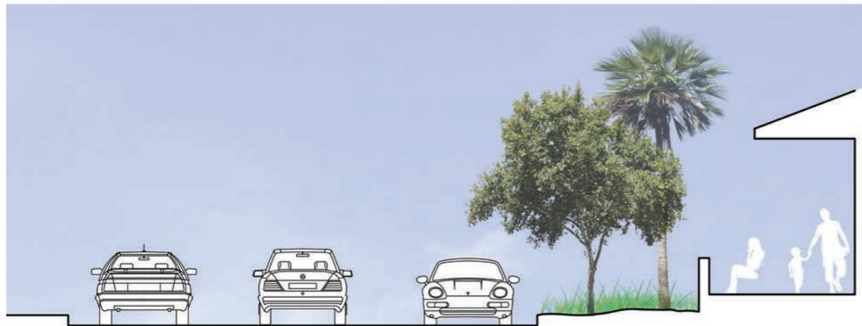
INDICATIVE MAIN STREET SECTION- PROPOSED- EAST END OF STREET (NO PARKING TO SOUTH SIDE OF STREET, KERB EXTENDED TO ALLOW FOR IMPROVED STREET AMENITY AND LANDSCAPE, IMPROVED OUTDOOR DINING)
