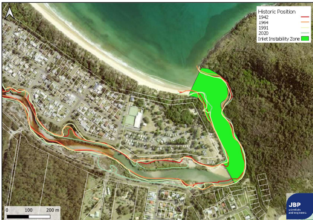
Figure 5-2: Entrance instability zone at Korogoro Creek, Hat Head
