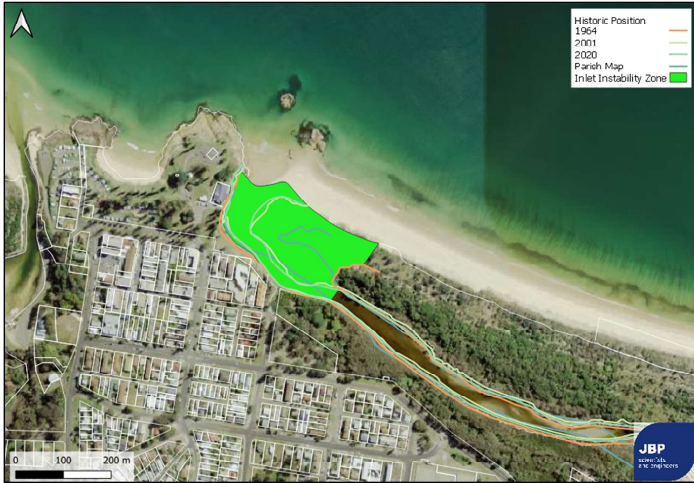
Figure 5-3: Entrance instability zone at Saltwater Creek
