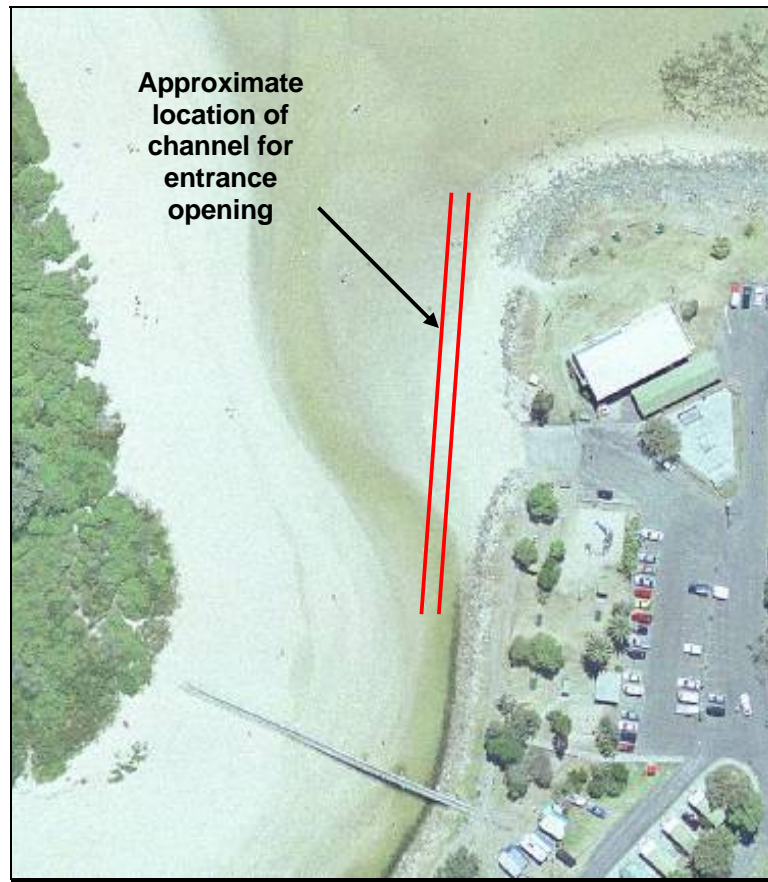
Figure A-3 Approximate position of pilot channel for inducing artificial breakout
